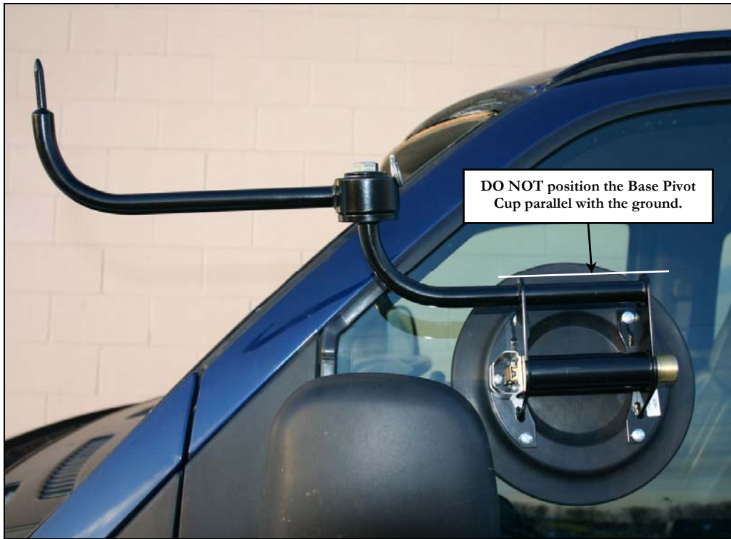
FIGURE 2 – Incorrect Base Pivot Cup Installation
