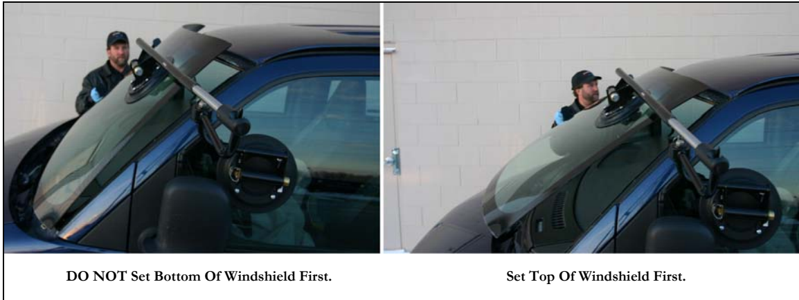
FIGURE 11 - Incorrect / Correct Windshield Installation
